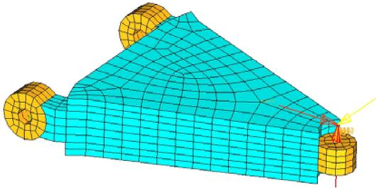
The orange areas are the inner pivot points and ball joint connections which are fixed by the suspension geometry and can't be changed, while the blue part is a solid volume of material that the software is allowed to cut away. There's also 3 separate loads applied to the part to represent braking, cornering, and hitting a pothole.
